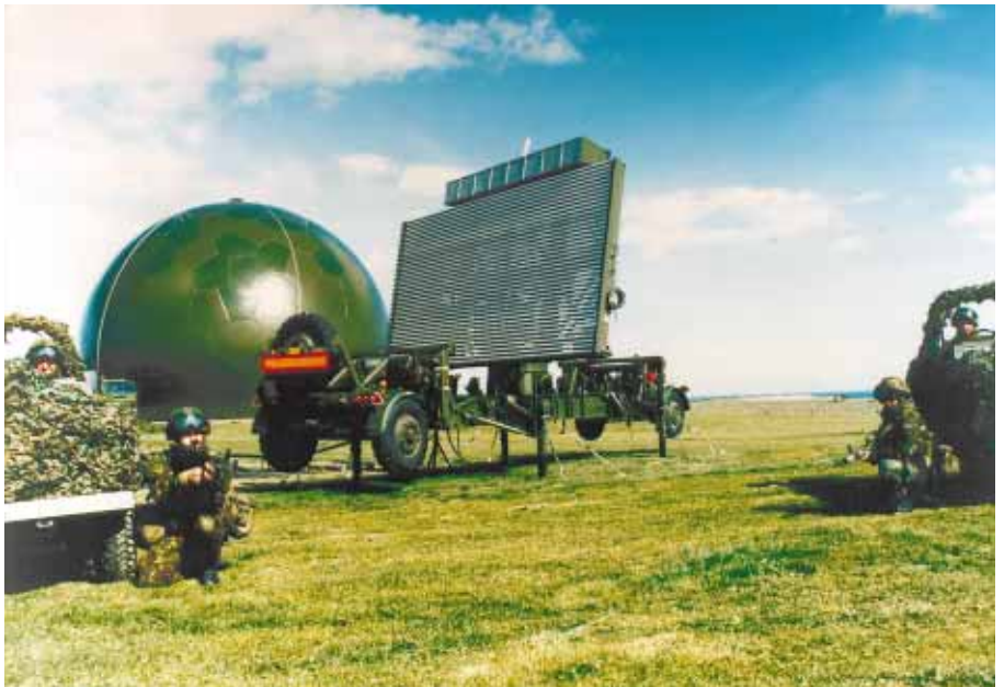
Siemens Plessey Systems' AR327 Commander tactical long-range air defense radar undergoing field testing
