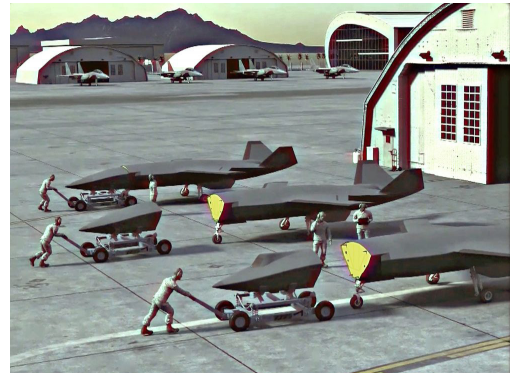
An animation from Roper's presentation shows digital Airmen preparing to switch nose cone sections on a notional modular unmanned aircraft. USAF
