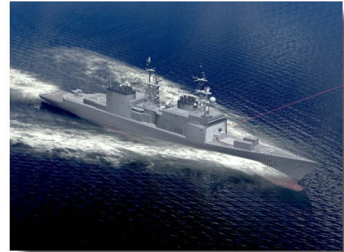
Artist's conception of the laser-armed U.S. Navy Self Defense Test Ship, nee USS Paul F. Foster (DD 964). Image source: Northrop Grumman .
