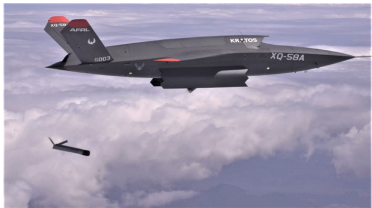
Kratos XQ-58A Valkyrie Successfully Completes Sixth Flight, Including First Payload Release from Internal Weapons Bay
