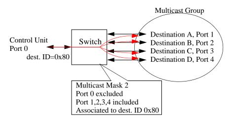
Figure 2-3. Multicast Configuration Example
