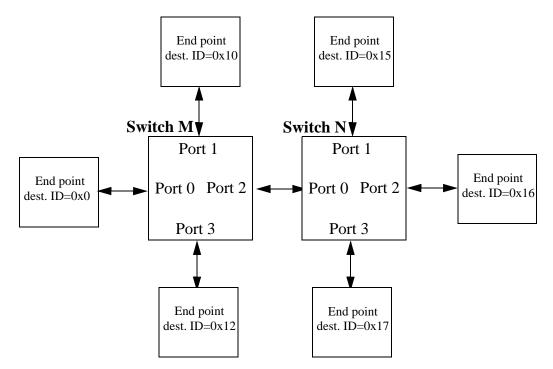
Figure 2-1. Multicast System Example
