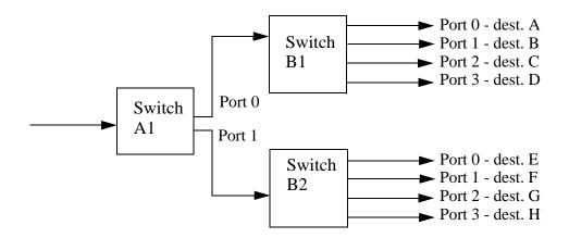
Figure 4-1. Example System using Multicast
