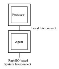
Figure 2-5. Processor-Only Processing Element Example
