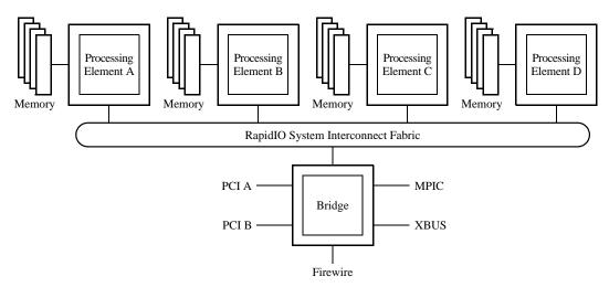
Figure 2-1. A Possible RapidIO-Based Computing System
