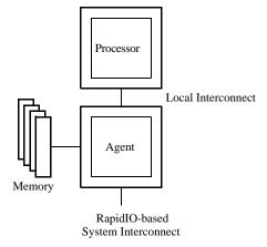
Figure 2-2. Processor-Memory Processing Element Example
