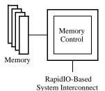
Figure 2-4. Memory-Only Processing Element Example
