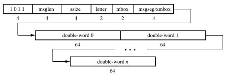
Figure 4-2. Type 11 Packet Bit Stream Format
