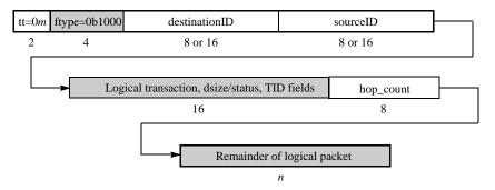
Figure 2-4. Maintenance Packet Transport Bit Stream
