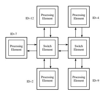
Figure 2-1. A Small Switch-Based System
