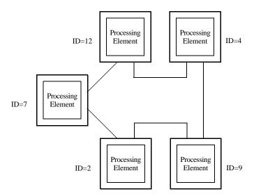
Figure 2-2. A Small Ring-Based System
